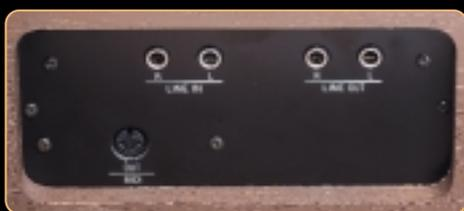
The New Hammond B-3 has a MIDI OUT jack which is located underneath the organ on the left side. To control another MIDI instrument (synthesizer,
